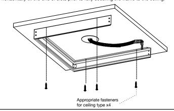
5.Put the wire conduit hose as close as possible to the surface mount opening before placing/inserting the luminaire into it partially. Make all electrical connections according to local code and make sure wire conduit hose is long enough for wiring connection job.
