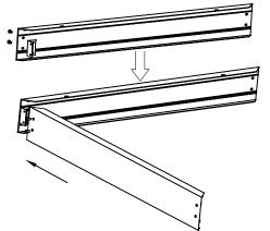
${\hbox{2.Repeat the previous step to secure the third mounting bracket.}}\\$
