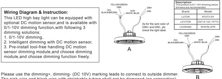
The pink wire and black wire with shrinkable tubing shall not be damaged (no connection). Class 1 Wiring Only.
